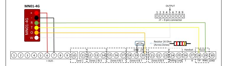
**NEW FEATURE:** For MiNi01-4G-V2, the status of the panel can be retrieved not only from the status PGM but now also from the Open/Close reports from the dialer. Therefore, wiring the white wire and programming of the status PGM of the panel is optional.
